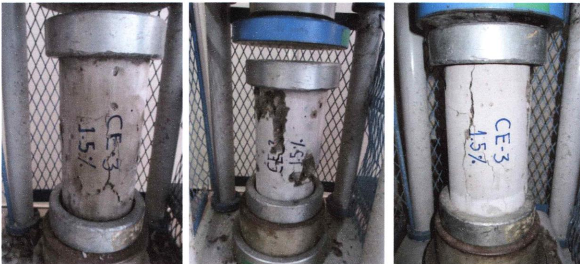
Concreto experimental 3 - 1.5 % SiO 2
